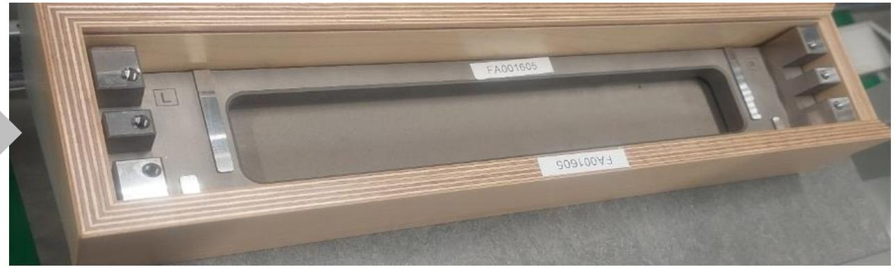
EOS M400-4 Recoater Blade Set up Fixture
