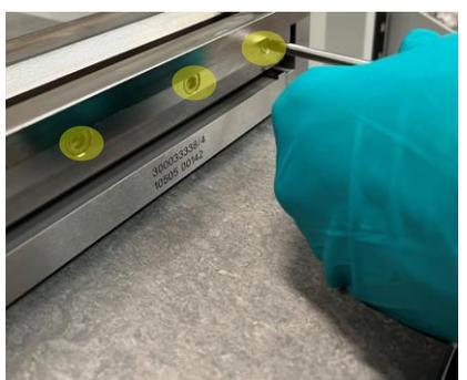
Bolt removal from the EOS M400-4 Recoater Blade Housing
