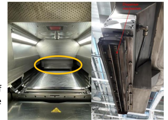
EOS M400-4 – Powder Dosing system located at the base of the hopper
